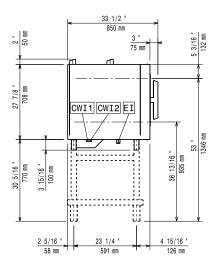
Cold Water inlet 1 CWI2 Cold Water Inlet 2
